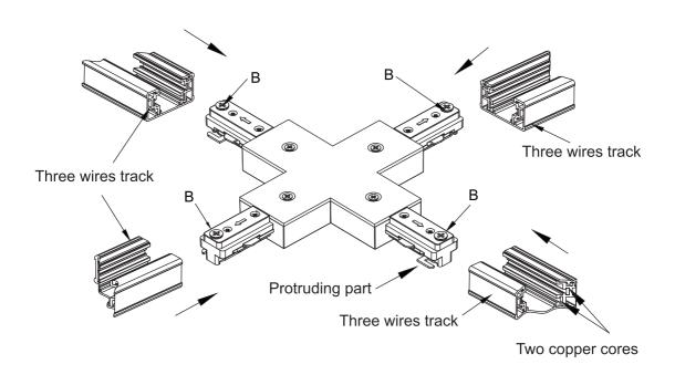
Loosen 4 screw-B on the X track rail connector, then insert the three-wire tracks into the connector following the arrow direction, and finally tighten all screw-B.
