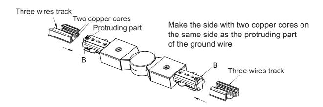
Loosen the 2 screws B on the three-wire angle connector first, then insert the three-wire tracks into the connector in the direction of the arrow, and finally tighten the screws B
