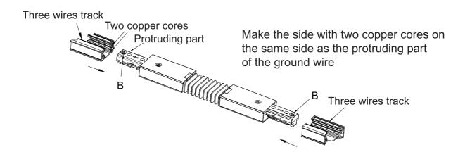
Loosen the 2 screws B on the three-wire fiexible connector first, then insert the three-wire tracks into the connector in the direction of the arrow, and finally tighten the screws B
